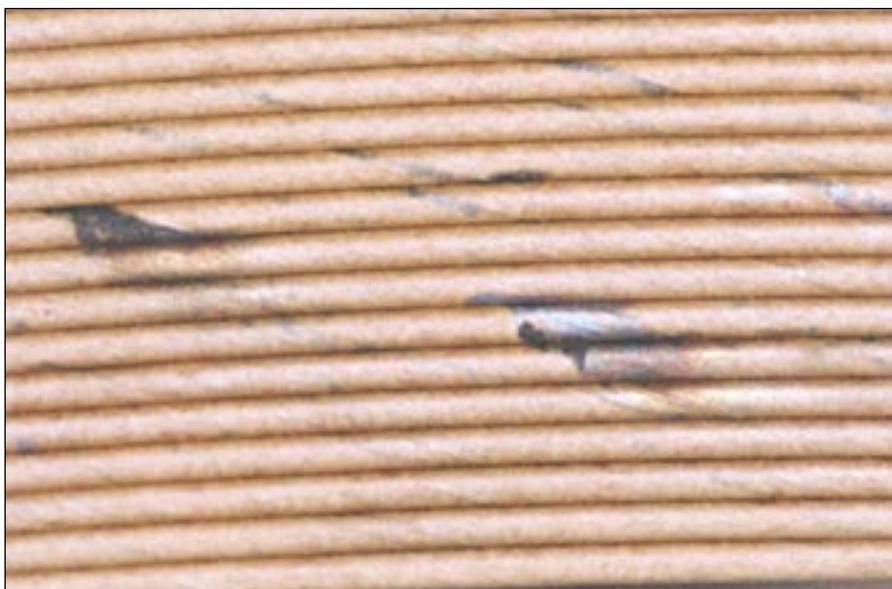
Fig. 1: Example of copper sulphide growing through several layers of covering paper.
