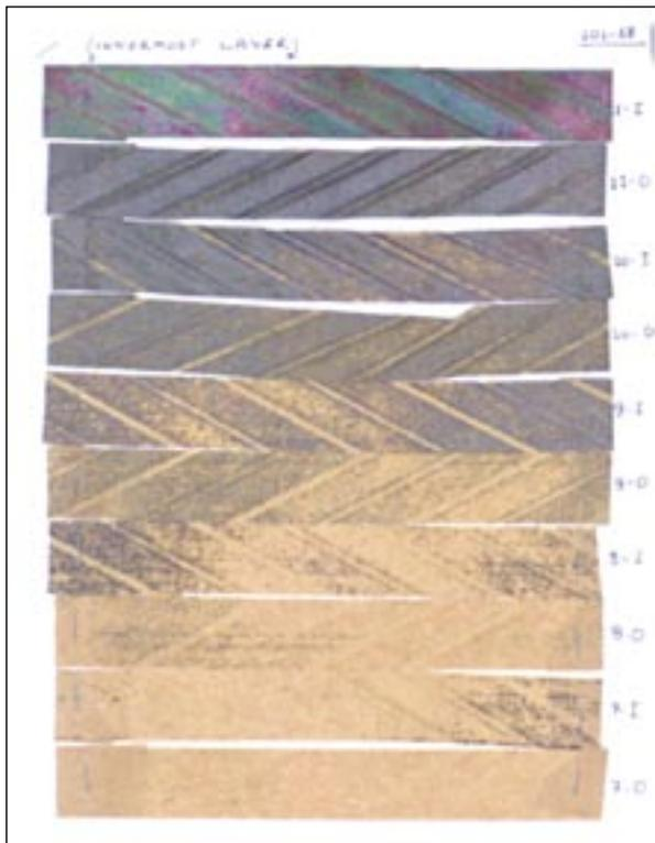
Fig. 2: Different layers (both sides shown) of covering paper from a conductor with varying degree of copper sulphide deposition.
