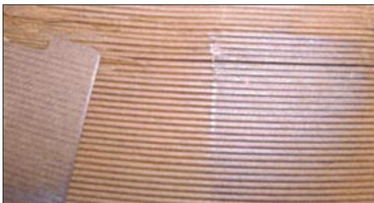
Fig.3: Example of copper sulphide deposited on spacer and under spacer. Similar deposits may also sometimes be seen on the outside of conductors in the area between the spacers.
